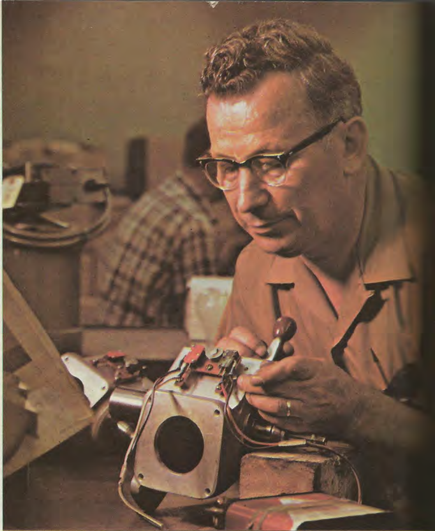
Broad range of attachments and accessories enhances overall utility of basic machine. Here contact points are adjusted in power feed unit
